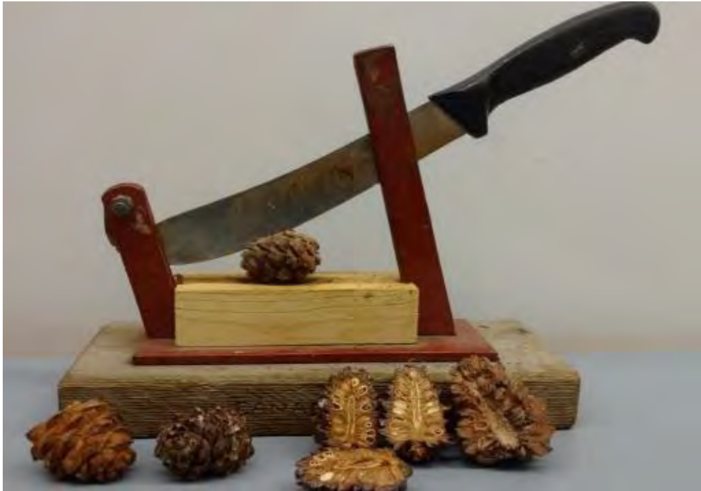
Figure 35. Cone knife used to evaluate the number of filled seeds and seed maturity.
